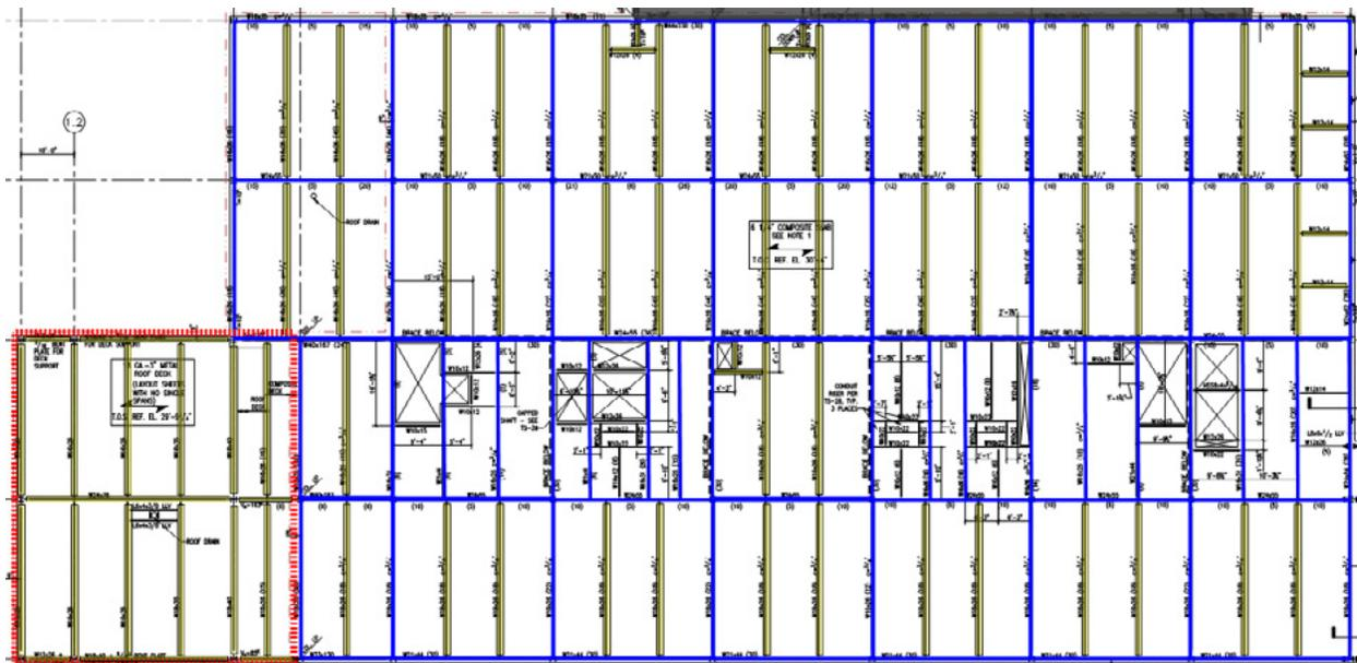
Figure 7-46. Design 3 Structural insulation distribution (Level 3 framing).
