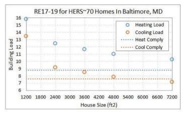
Notes: Insulation values approximately equal to 2012 IECC. HERS Index score of 70 based on RESNET/ICC 301. None of these homes fully comply with RE17-19, but it's clear that larger homes will have an easier time complying than smaller homes.
