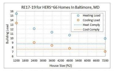
Notes: Insulation and air leakage values in compliance with 2018 IECC. Standard efficiency equipment. HERS Index in accordance with RESNET/ICC 301. No homes fully comply, but it's clear that larger homes will have an easier time complying than smaller ones.
