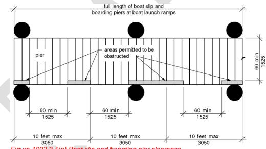
Figure 1003.3.1(a) Boat slip and boarding pier clearance
