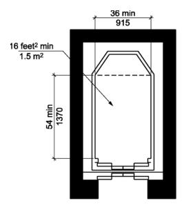
(e) Existing Car Configurations e) existing car configuration
