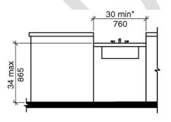
\* 36 in. (915 mm) min. if part of T-shaped turning space per Sections 304.3.2 and 1003.3.2 *Figure 1103.12.4 - Kitchen sink for Type A units*
