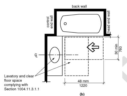
Figure 1104.11.3.1.3.1(a&b) - Parallel approach bathtub in Type B units – Option A bathroom
