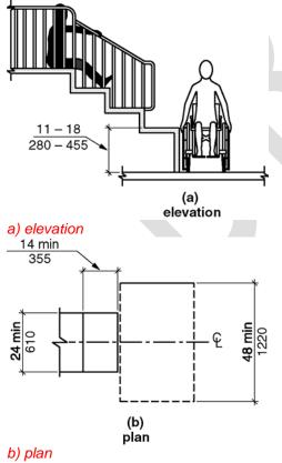
**1008.4.2.1.1 Size.** Transfer platforms shall have level surfaces 14 inches (355 mm) minimum in depth and 24 inches (610 mm) minimum in width.
