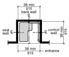
Note: inside finished dimensions measured at the center points of opposing sides *Figure 608.2.1.1 – Transfer type shower compartment size*
