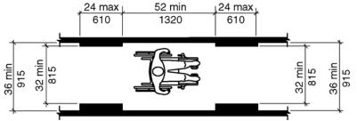
Figure 403.5.1(a)- Clear width of an accessible route - new buildings and facilities - interior
