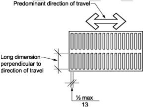
Figure 302.3 Openings in floor surface
