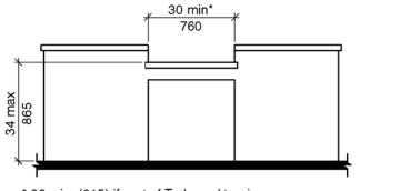
\* 36 min. (915) if part of T-shaped turning space per Sections 304.3.2 and 1003.3.2 Figure 1103.12.3 – <u>Accessible Work surface in kitchen for Type A units</u>
