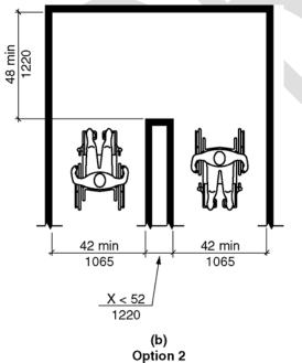
Figure 403.5.2.1(b) - Clear width at 180 degree turn – new buildings and facilities – Option 2
