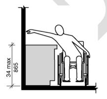
**Height** Figure 1104.11.3.2.1 - Lavatory in Type B units – Option B bathroom
