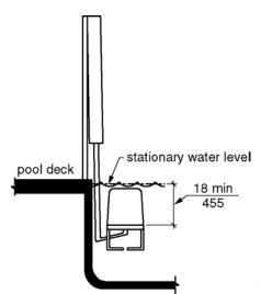
Figure 1009.2.8 - Pool lift submerged depth
