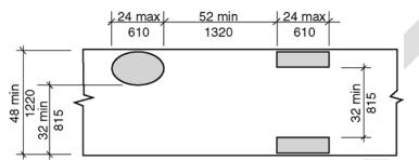
Figure 403.5.1(b) - Clear width of an accessible route - new buildings and facilities - exterior
