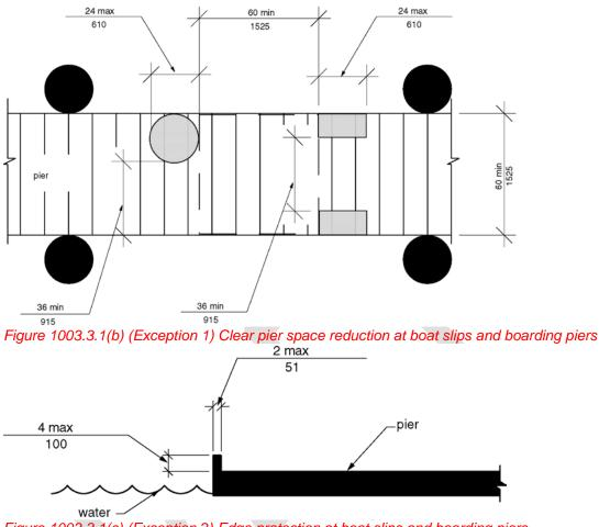
Figure 1003.3.1(c) (Exception 2) Edge protection at boat slips and boarding piers
