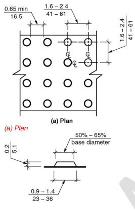
(b) Elevation (Enlarged) (b) Elevation (enlarged)
