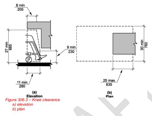
**306.3.1 General.** Space beneath an element between 9 inches (230 mm) and 27 inches (685 mm) above the floor shall be considered knee clearance and shall comply with Section 306.3.
