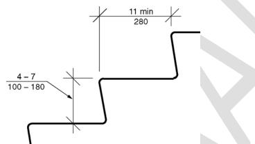
Figure 504.2 - Treads and risers for stairways
