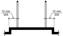
Figure 405.9.1 Extended floor surface
