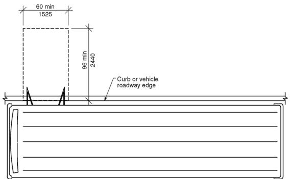
Figure 805.2.2(b) - Size of bus boarding and alighting area- existing buildings and facilities
