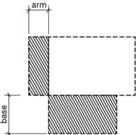
Figure 304.3.2.2(b) T-shaped turning space – existing buildings and facilities – overlap
