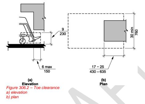
**306.2.1 General.** Space beneath an element between the floor and 9 inches (230 mm) above the floor shall be considered toe clearance and shall comply with Section 306.2.
