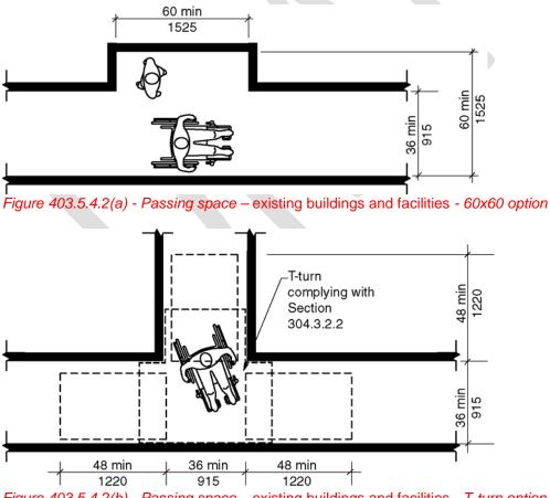
Figure 403.5.4.2(b) - Passing space – existing buildings and facilities - T-turn option
