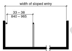
Figure 1009.3.3 - Handrails for sloped entry
