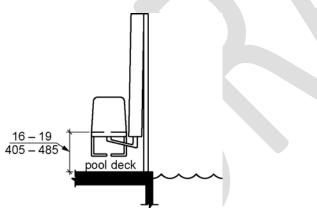
Figure 1009.2.4 - Pool lift seat height
