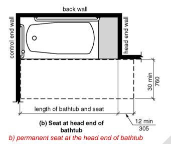
**607.3 Seat.** A permanent seat at the head end of the bathtub or a removable in-tub seat shall be provided. Seats shall comply with Section 610.
