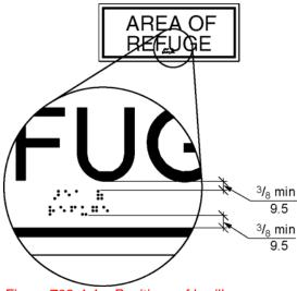
Figure 703.4.4 – Positions of braille
