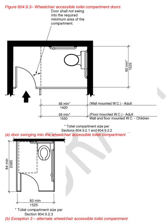
**604.9.3.1 Door Opening Location.** The farthest edge of the wheelchair accessible toilet compartment door opening shall be located in the front wall or partition or in the side wall or partition as required by Table 604.9.3.1.
