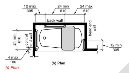
**607.4.2.1 Back Wall.** Two horizontal grab bars shall be provided on the back wall, one complying with Section 609.4 and the other located 8 inches (205 mm) minimum and 10 inches (255 mm) maximum above the rim of the bathtub. Each grab bar shall be 24 inches (610 mm) minimum in length, located 24 inches (610 mm) maximum from the head end wall and extend to 12 inches (305 mm) maximum from the control end wall.
