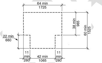
Figure 304.3.2.1(b) T-shaped turning space- new buildings and facilities - Option 2
