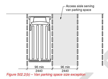
**502.3 Vehicle Space Marking.** Car and van parking spaces shall be marked to define the width. Where parking spaces are marked with lines, the width measurements of parking spaces and adjacent access aisles shall be made from the centerline of the markings.
