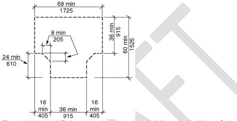
Figure 304.3.2.1(a) T-shaped turning space- new buildings and facilities - Option 1
