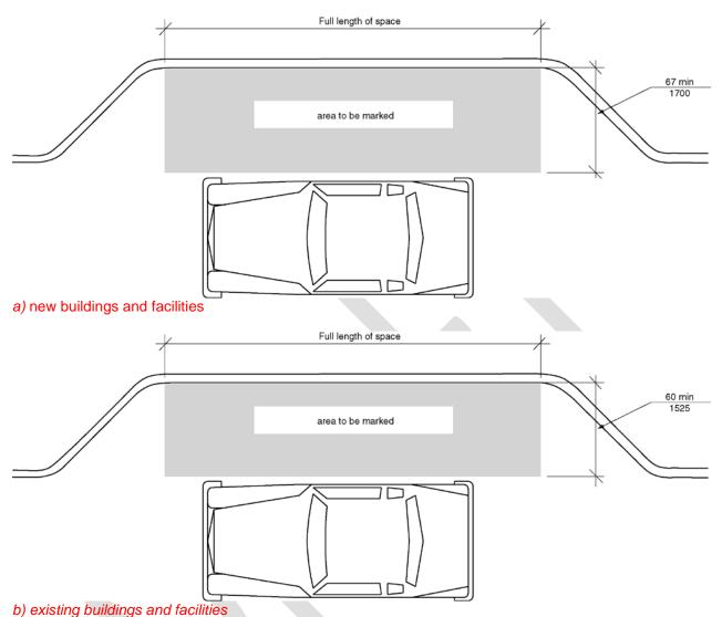
Figure 503.3 (a) and (b) - Passenger loading zone access aisle
