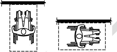
**Figure 305.5** Position of clear floor space a) forward b) parallel
