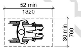
Figure 305.3.1 - Size of clear floor space - new buildings and facilities
