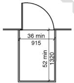
Figure 410.5.1.1 lifts with single door or opposite end door – new buildings
