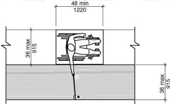
Note: Running Slope of Clear Floor or Ground Space Not Steeper Than 1:20 b) existing buildings and facilities
