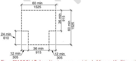
Figure 304.3.2.2(a) T-shaped turning space – existing buildings and facilities – size
