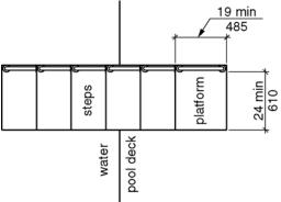
Figure 1009.5.1 - Size of transfer platforms
