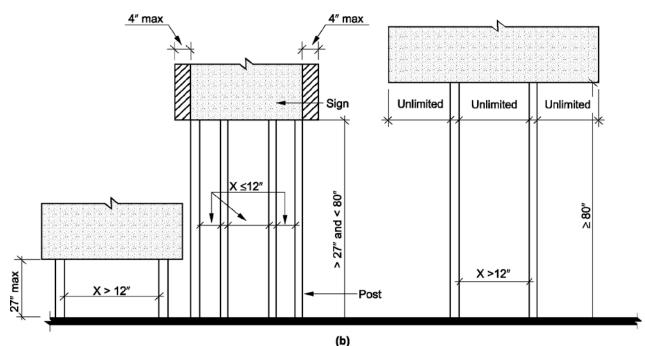
Figure 307.3 (a)&(b) Post-mounted protruding objects
