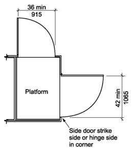
(b) Platform with doors on adjacent sides b) platform with doors on adjacent sides
