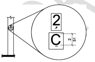
Figure 407.2.3.2 - Destination-oriented elevator car identification
