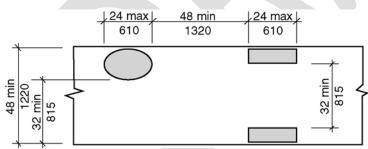
Figure 403.5.1(d) - Clear width of an accessible route - existing buildings and facilities - exterior
