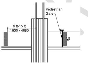
Pedestrian At-Grade Rail Crossing Figure 705.7.5 – Pedestrian at-grade rail crossings
