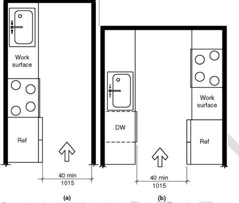
Figure 1103.12.1.1 (a&b) Minimum kitchen clearance in Type A units
