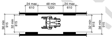
Figure 403.5.1(c) - Clear width of an accessible route - existing buildings and facilities - interior
