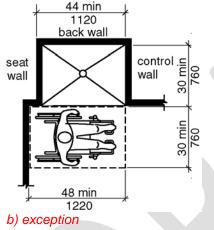
**1104.11.3.2 Option B.** One of each type of fixture provided shall comply with Section 1104.11.3.2. These fixtures shall be in a single toilet/bathing area, such that travel between fixtures does not require travel through other parts of the unit.
