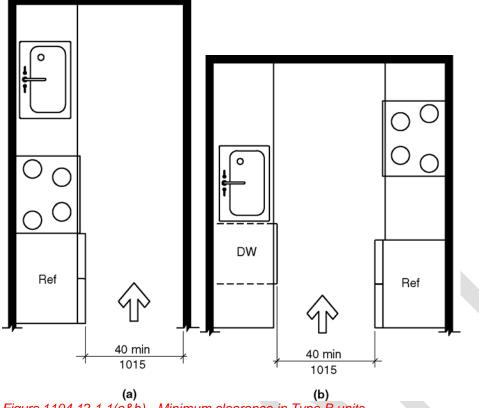
Figure 1104.12.1.1(a&b) - Minimum clearance in Type B units
