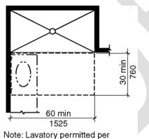
Section 608.2.2 Figure 1103.11.2.5.2 Standard roll-in-type shower compartment in Type A units
