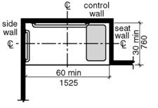
Note: inside finished dimensions measured at the center points of opposing sides *Figure 608.2.2.1 - Standard roll-in-type shower compartment size*
