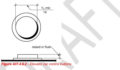
**407.4.6.2.1 Size.** Buttons shall be <sup>3</sup>/<sub>4</sub> inch (19 mm) minimum in their smallest dimension.
