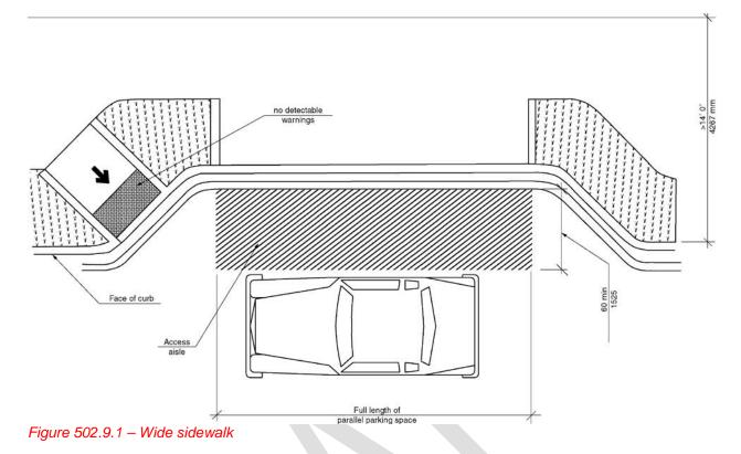
**502.9.1.1 Alterations.** In alterations where the street or sidewalk adjacent to the parking spaces is not altered, an access aisle shall not be required provided the parking spaces are located at the end of the block face.
