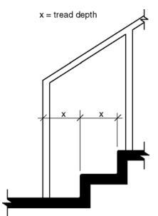
Figure 505.10.3 - Bottom handrail extensions at stairs
