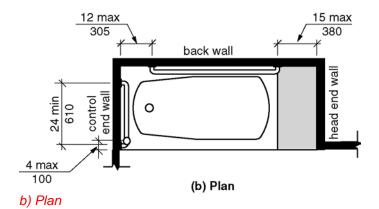
**607.4.1.1 Back Wall.** Two horizontal grab bars shall be provided on the back wall, one complying with Section 609.4 and the other located 8 inches (205 mm) minimum and 10 inches (255 mm) maximum above the rim of the bathtub. Each grab bar shall be located 15 inches (380 mm) maximum from the head end wall and extend to 12 inches (305 mm) maximum from the control end wall.
