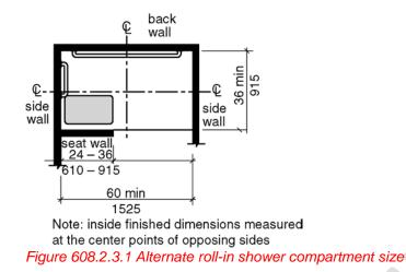
**608.2.3.2 Seat.** A folding seat complying with Section 610 shall be provided on the seat wall opposite the back wall.
