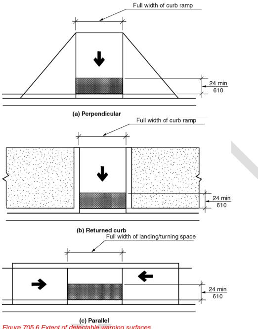
Figure 705.6 Extent of detectable warning surfaces a) perpendicular b) returned curb c) parallel
