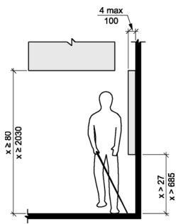
Figure 307.2 Limits of protruding objects
