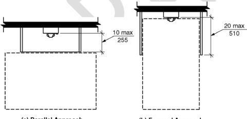
(a) Parallel Approach (b) Forward Approach Figure 704.2.1 - Clear floor space for telephones
