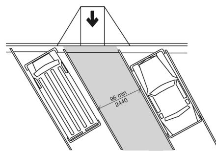
Figure 502.9.2 - Perpendicular or Angled Parking Spaces
