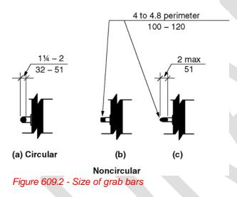
**609.2.1 Circular Cross Section.** Grab bars with a circular cross section shall have an outside diameter of  $1^{1}/_{4}$  inch (32 mm) minimum and 2 inches (51 mm) maximum.
