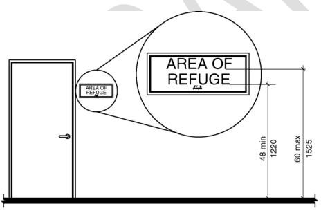
Note: For braille character mounting height see Section 703.4.5 Figure 703.3.10 – Height of raised characters above floor
