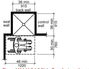
Figure 1104.11.3.1.3.3(a) - Transfer type shower compartment in Type B units
