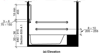
Figure 607.4.1 (a) and (b) Grab bars for bathtubs with permanent seats at head end of bathtub
