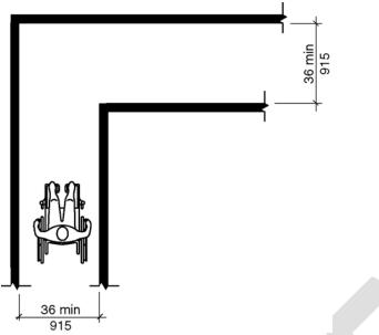
Figure 403.5.3.2 - Clear width at 90 degree turn – existing buildings and facilities
