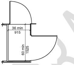
**410.5.2.1 New buildings.** In new buildings, platform lifts with doors on adjacent sides shall provide a clear floor width of 42 inches (1065 mm) minimum and a clear floor depth of 60 inches (1525 mm) minimum.
