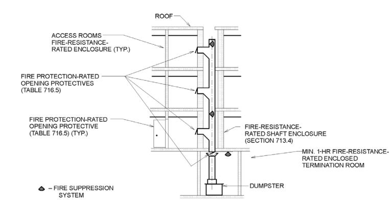
In Figure 713.13.3 REFUSE CHUTE (FIRE BARRIER OPTION), replace the right hand note as follows: MIN. 1-HR FIRE-REISTANCE-RATED ENCLOSED TERMINATION ROOM. FIRE-RESISTANCE RATED EQUAL TO THAT REQUIRED FOR THAT SHAFT ENCLOSURE.
