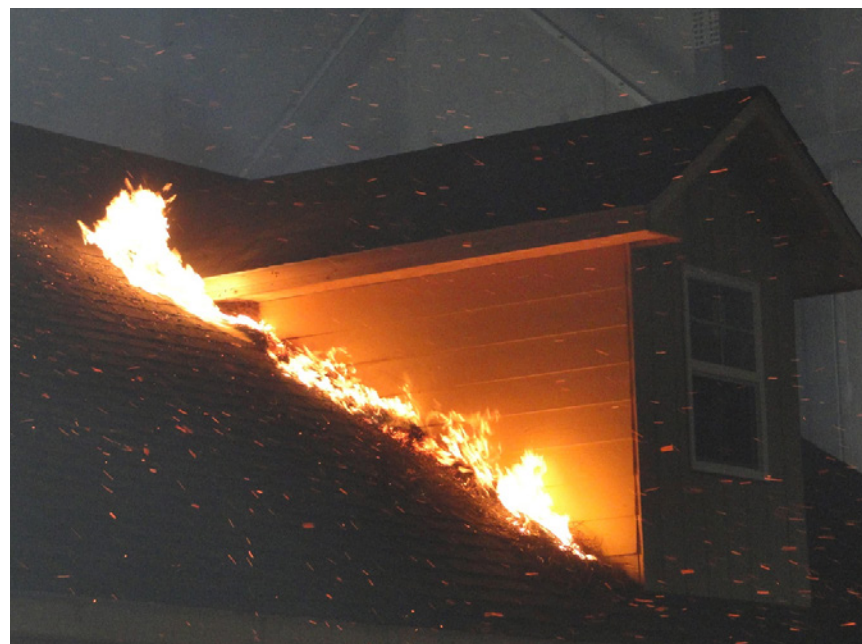
Ember-ignited debris results in flame contact to the siding and soffit area on this dormer during testing at the IBHS Research Center in 2011.
